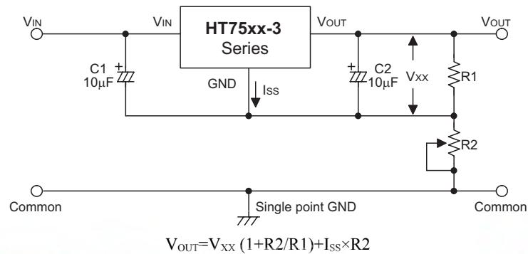
**Circuit for Increasing Output Voltage**
